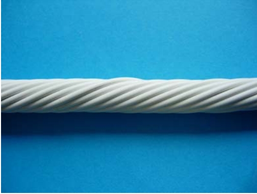
NOT ACCEPTABLE Lay length too short (Cable over twisted)
