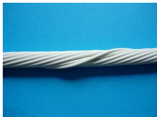
NOT ACCEPTABLE Wire crossing over
