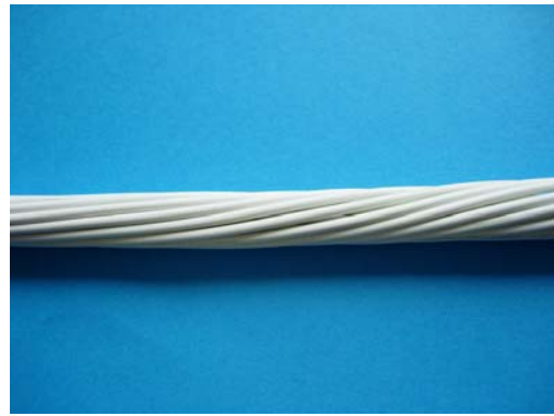
NOT ACCEPTABLE Lay length too long (Cable under twisted)
