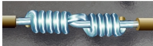
Figure 19-16. Completed Wrap for Western Union/Lineman Splice
