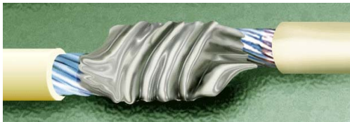
Figure 19-10. Soldered Lash Splice
