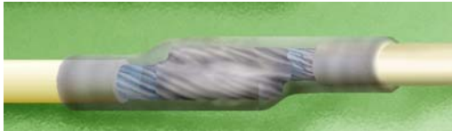
Figure 19-3. Sleeving over Soldered Connection
