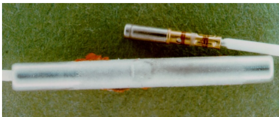
Figure 19-32. Crimped Contact Outside Junction Device
