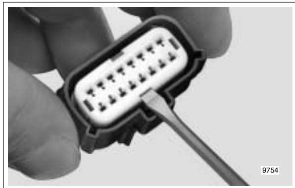
Figure B-43. Pry Up Secondary Lock (Socket Housing)
