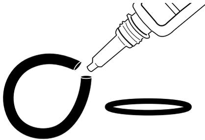
1. Cut the starting end of the cord stock with a clean razor blade. Ensure the cut is clean and square. Do not touch the clean cut end.
