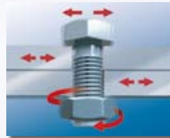
Vibration and loosening
