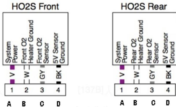
**Installation: Dual O2 Wiring Sequence: 8 Wires**
