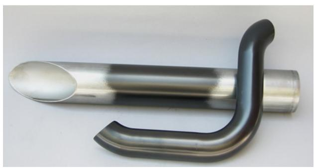
Here the part has had a simple single coat and the surface has been rubbed with a clean white cloth. A Black Ceramic Heat Shield is provided as a comparison.
