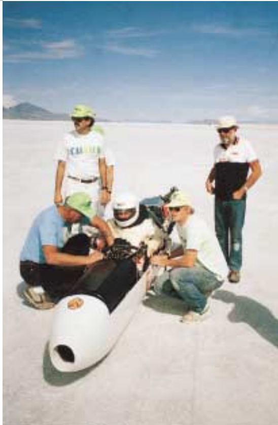
Above: Besides a fireproof suit, the SCTA requires drivers to wear fireproof boots and gloves, a helmet, a neck brace (here being adjusted by Joe Von Harten), and wrist restraints to keep your arms safely inside the roll cage in the event of a crash. Right: You don't sit down in a streamliner as much as put it on. Clockwise from left: Von Harten helps Wheeler with the seven-point safety harness (another SCTA requirement), while Andrews (standing in front of his wife, Jill), Frank Sherrill, and Moore stand by.
