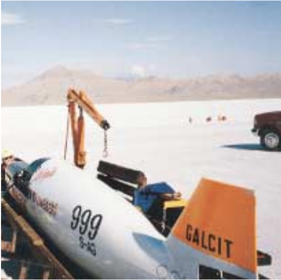
Moore checks the tail fin's alignment. The fin, which was damaged in the crash, eventually had to be rebuilt completely; sadly, only one set of GALCIT decals had been made.
