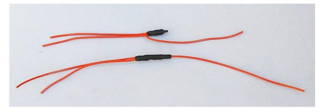
The Parallel Stub Splice has all three wires in one end and one wire loops back. This method results in the shortest splice and the best stress relief and has 3/4" of adhesive heat shrink
