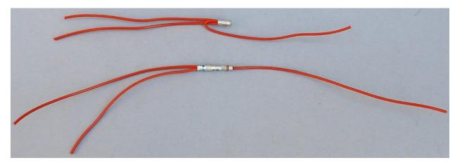
Top splice is a Parallel Stub Splice
