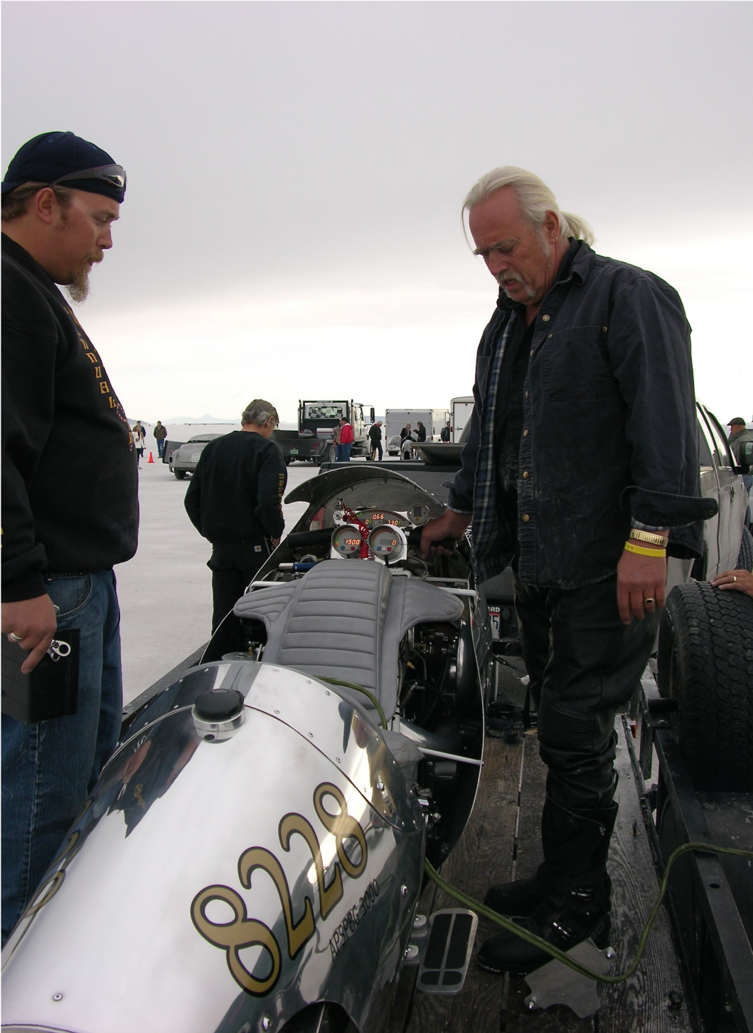
Warming the bike up before the start. Bryan getting ready to leave down a wet slippery course. During the run there was a fuel delivery problem and the engine lost power. Turns out it was a clogged filter from some metal shavings left a decade ago in the baffles of the custom made stainless fuel tank. The engine had to come apart.
