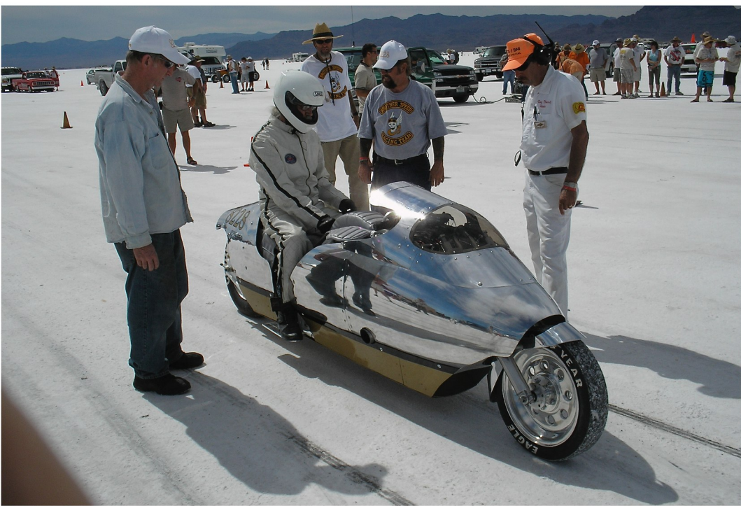
Bonneville Speed Week 2008. Mike Geokan and his 17 year odyssey are about to leave the starting line. The engine has run a total of less than 10 minutes and the bike has never been ridden, much less turned a wheel, beyond rolling to the starting line. 1000 lbs, 45 degrees of rake, up to 425 hp, an untested clutch, and Mike.
