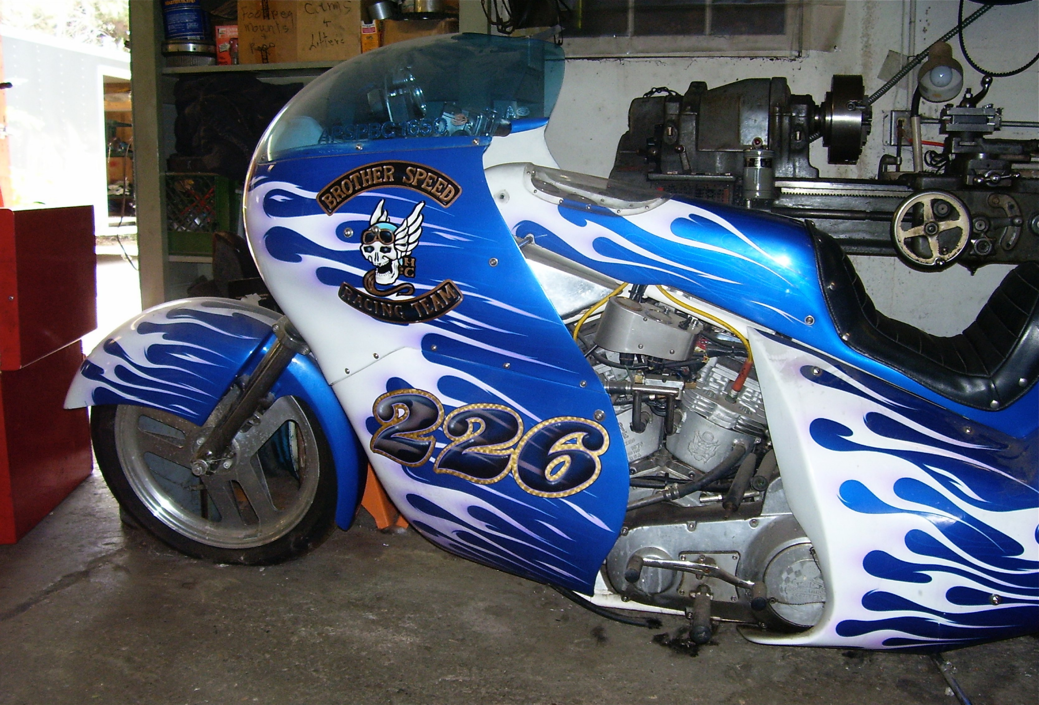
Retired #226 Blue Bike. Designed and built by Mike. Bonneville record holder for over a decade. Watercooled, turbocharged, intercooled, fuel and water injected 104" Evo engine. Angry, she watches the Bullet come to life.
