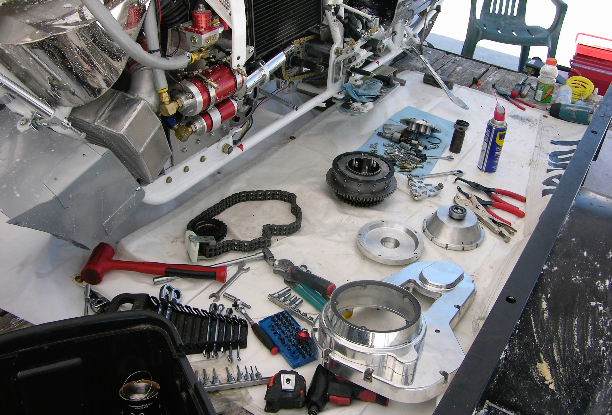
Bryan pulled the primary, clutch, and transmission and Carl Pelletier had transmission tools and parts sent Next Day Air to the salt. Other parts were driven in from Salt Lake City. Bryan had to grind a bearing race off of the main shaft. Repaired, the bike ran 174 and 183 mph in the two mile. If you don't run, you don't sort it out.
